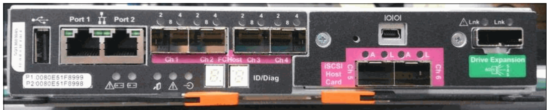
Figure 1-11 Controller module with an optional iSCSI host interface daughter card
