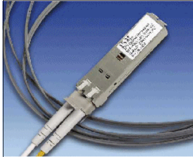
Figure 2-5 Small Form Pluggable (SFP) with LC connector fiber cable
