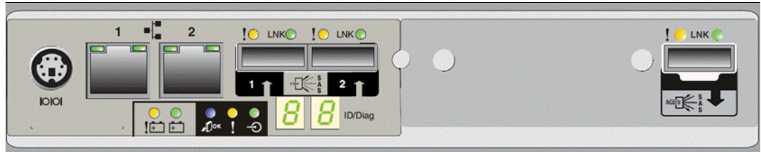
Figure 3-1 The rear panel of a DCS3700 controller
