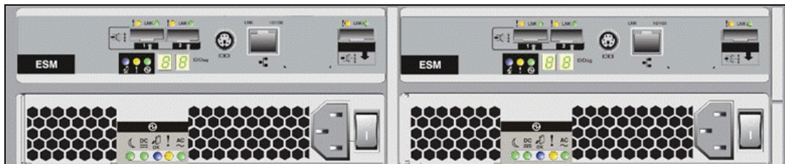
Figure 3-6 The rear panel of a DCS3700 expansion unit.
