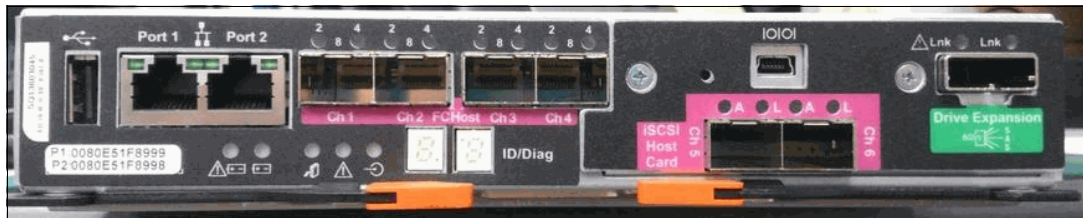
Figure 3-5 Controller module with an optional iSCSI host interface daughter card
