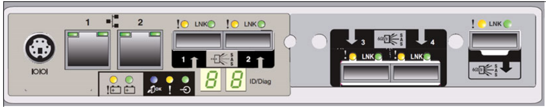
Figure 3-2 The rear panel of a DCS3700 controller with the optional SAS host port adapter installed
