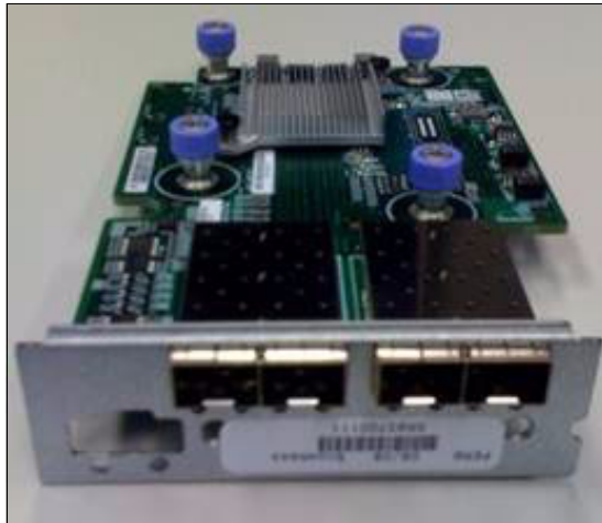
Figure 1-8 Example host interface daughter card module
