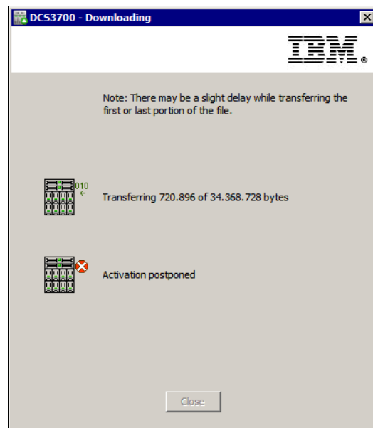
Figure 14-36 Downloading the firmware with activation postponed
